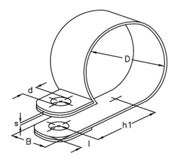
$\begin{array}{ll} d & = 5.3 \\ \text{Diameter D} = 47 \\ \text{h1} & = 30.3 \\ \text{I} & = 5.0 \\ \text{s} & = 0.5 \\ \text{Width B} & = 12 \\ \end{array}$
